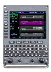
Flight Planning Made Easy Entering and editing Flight Plans has never been easier than with the Avidyne Atlas. It features easy-to-use flight planning with 'one-touch' victor airway and jet-route navigation, Avidyne's exclusive GeoFill™ waypoint nomination, and full autopilot integration.
