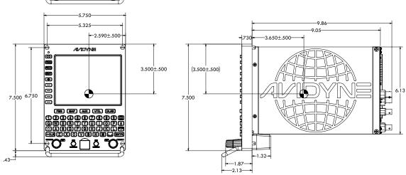
Designed to fit. Avidyne Helios packs all these capabilites in a standard dzus-mount design.
