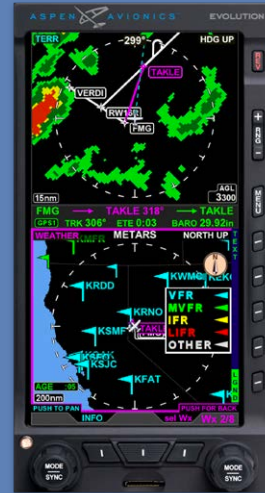
Easily zoom, pan, and see your present position overlaid on geo-referenced charts and airport diagrams. In flight, cross-check positioning between chart and moving map.
