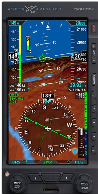
PFD display showing optional Synthetic Vision and Angle of Attack.
