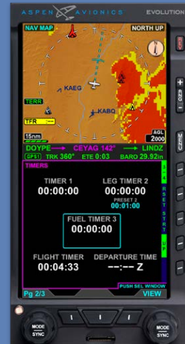
Easily zoom, pan, and see your present position overlaid on geo-referenced charts and airport diagrams. In flight, cross-check positioning between chart and moving map.
